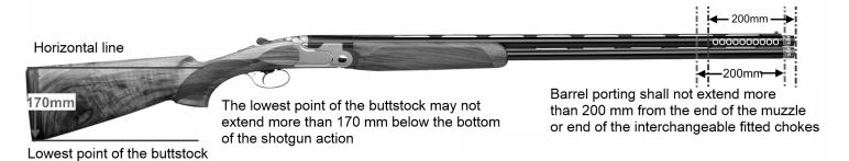
The lowest point of the buttstock or toe of the butt plate may not be more than 170 mm below a horizontal line extending from the bottom of the shotgun action (see illustration).
